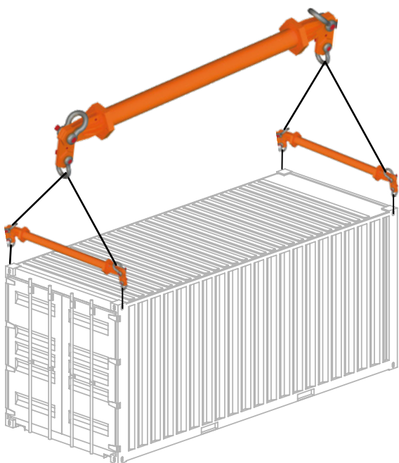
Lifting with vertical twistlocks.
